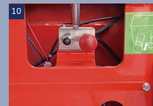
Manual release valve: When the machine can not move, you can push the machine after pressing this valve
