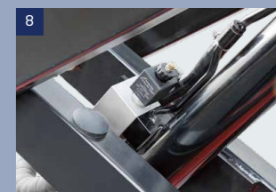
Explosion proof valve: To prevent the machine falling when the oil pipe is leaking
